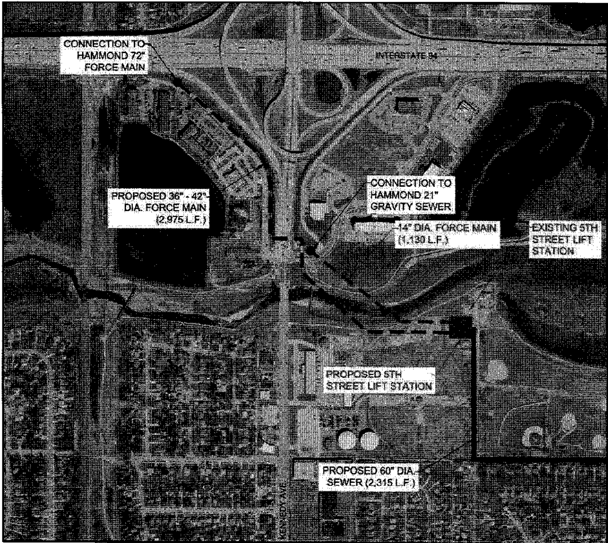
Figure 2 – SSO Remedial Project Phase 1 – Division B (Lift Station) & Division C (Force Mains) – General Site layout
